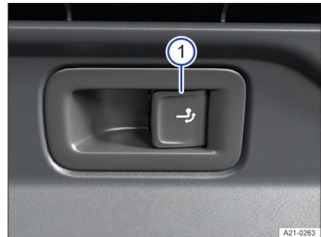
Fig. 190 On the right of the luggage compartment: button for releasing the ball coupling.
