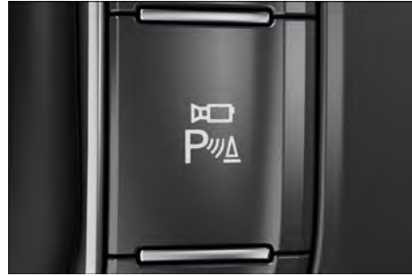
Fig. 163 In the centre console: button for switching Area View on and off.
