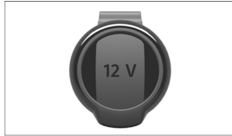
Fig. 172 In the front stowage compartment, in the rear centre console or on the left-hand side of the luggage compartment: fold-open 12-volt socket (illustration).
