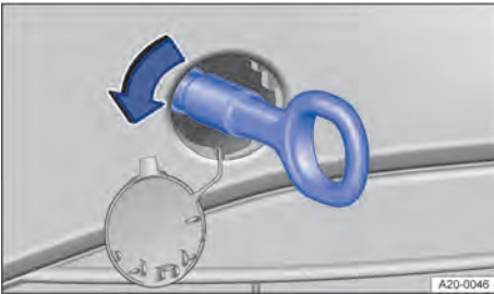
Fig. 224 In the front bumper on the right: screwing in the towing eye.
