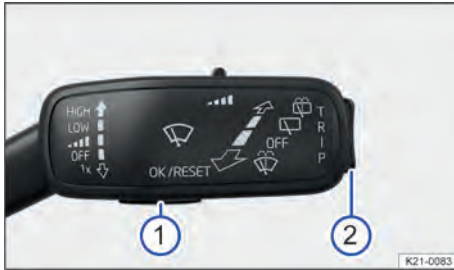
Fig. 17 On the right of the steering column: buttons on the wiper lever.
