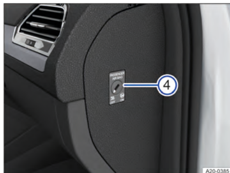
Fig. 9 With open front passenger door (left-hand drive vehicles): key-operated switch in the dash panel (mirrored for right-hand drive vehicles).
