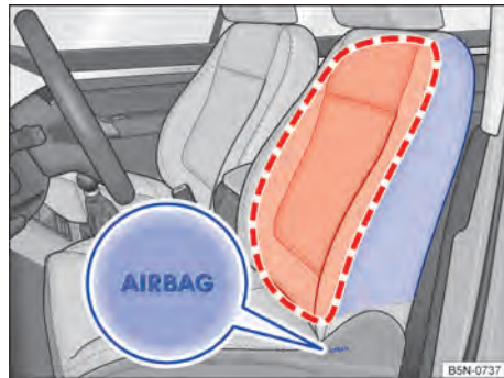
Fig. 44 On the side of the front seat: location and deployment zone of the side airbag.
