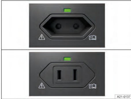
Fig. 173 In the luggage compartment on the left side: 230-volt socket, 115-volt socket or 100-volt socket.
