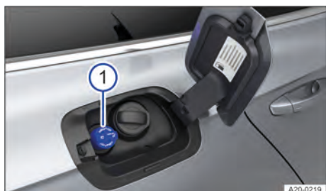
Fig. 200 Behind the tank flap: tank cap for AdBlue (illustration).
