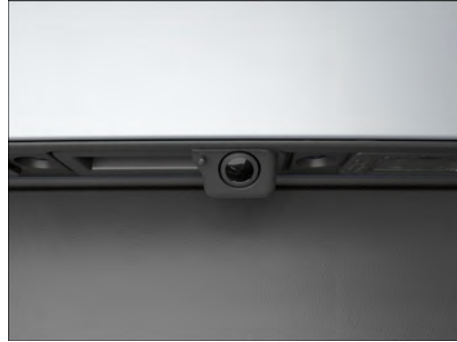
Fig. 261 At the rear of the vehicle: rear view camera system on the handle button (illustration).
