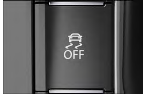
Fig. 169 In the centre console: button for switching TCS, ESC and ESC Sport on and off manually (with some equipment levels).
