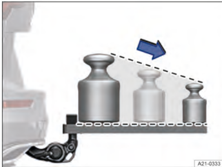
Fig. 192 Recommended weight distribution on the rear carrier system.
