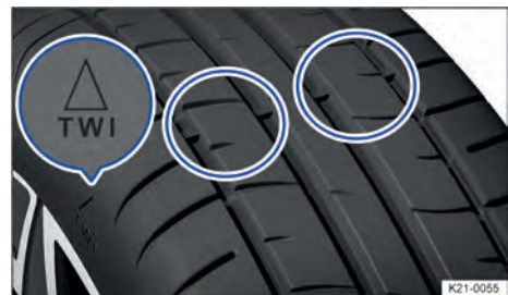
Fig. 244 Tyre tread: tread wear indicators.
