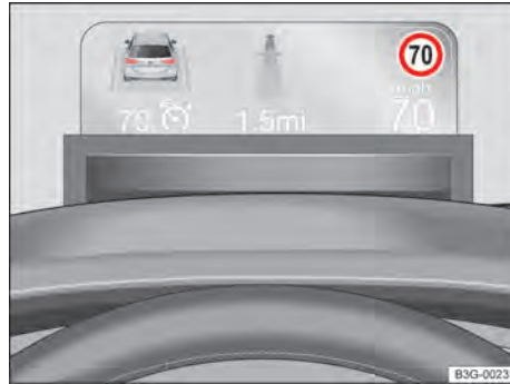
Fig. 23 On the dash panel above the steering wheel: examples of information shown in the Head-up Display.
