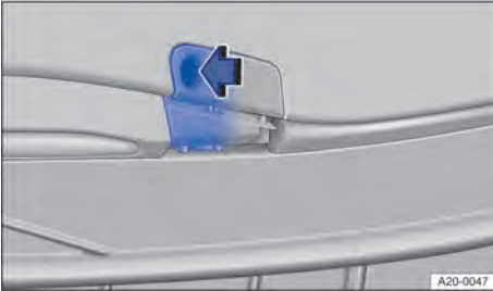
Fig. 223 In the front bumper on the right: removing the cover (R Line).
