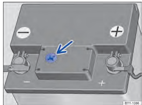
Fig. 239 Battery window on the top of the 12-volt vehicle battery (illustration).
