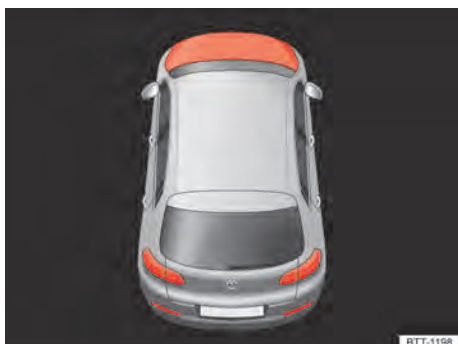
Fig. 230 On the instrument cluster display: the bonnet is open or not closed properly (illustration).
