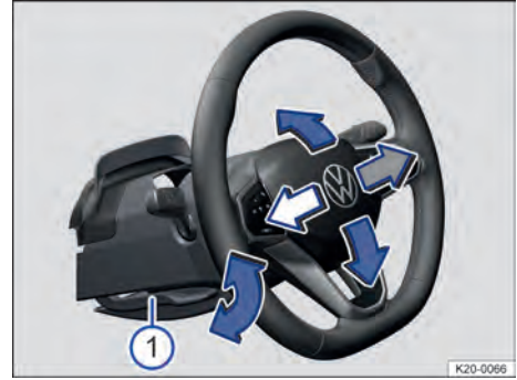
Fig. 75 Below the steering wheel in the steering column trim: lever for mechanical adjustment of the steering wheel position (illustration).
