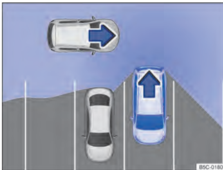
Fig. 167 Illustration of Rear Traffic Alert: monitored area around the vehicle leaving the parking space.
