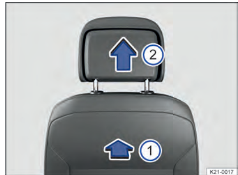
Fig. 89 Illustration: removing front head restraint.
