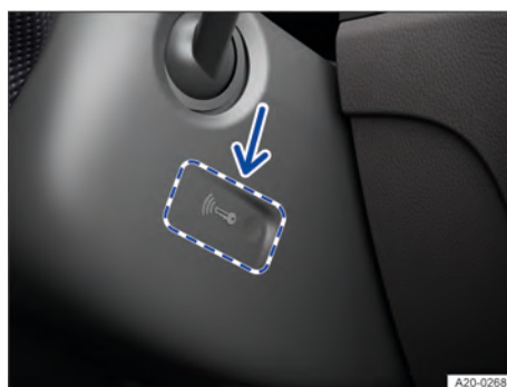
Fig. 121 On the right-hand side of the steering column: emergency start function in vehicles with the keyless locking and starting system Keyless Access.
