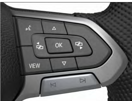
Fig. 15 Right-hand side of the multifunction steering wheel: buttons for using the menus and information displays in the analogue instrument cluster (variant 1).
