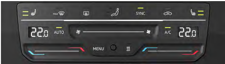
Fig. 110 In the upper part of the centre console: Climatronic air conditioning block.
