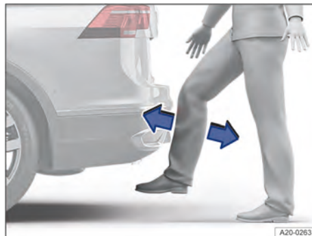
Fig. 70 Illustration of the boot lid with sensor-controlled closing (Easy Close).
