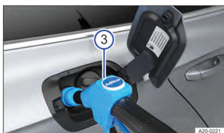
Fig. 202 Behind the tank flap: refilling AdBlue using the nozzle (illustration).
