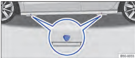
Fig. 254 Jacking points (illustration).
