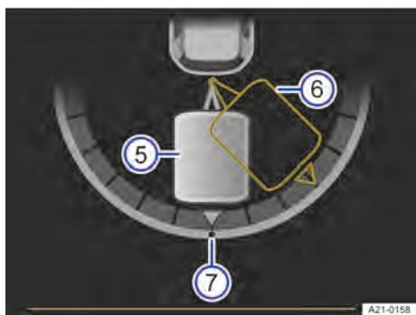
Fig. 166 In the instrument cluster display: adjusting the vehicle and trailer angle.
