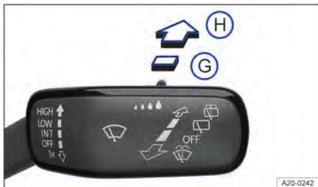
Fig. 102 On the right-hand side of the steering column: operating the rear window wiper.
