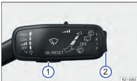
Fig. 13 On the right of the steering column: buttons on the wiper lever.
