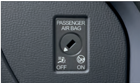
Fig. 42 In the dash panel on the front passenger side: key-operated switch for deactivating and activating the front airbag on the front passenger side
