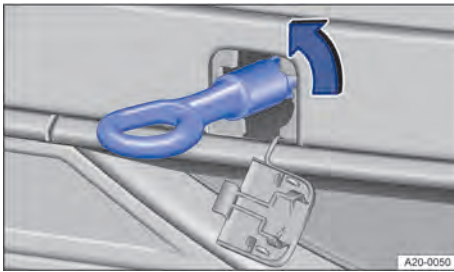
Fig. 227 In the rear bumper on the right: screwing in the towing eye.
