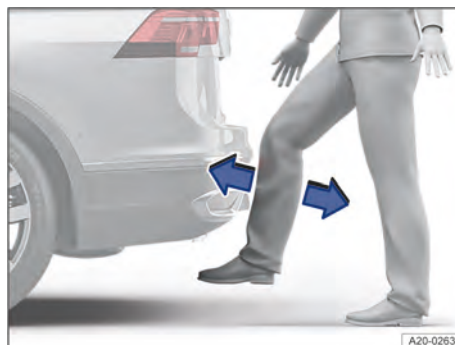
Fig. 69 Illustration of the boot lid with sensor-controlled opening (Easy Open).
