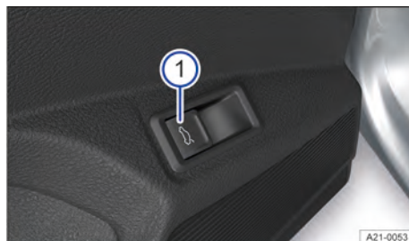
Fig. 60 In the driver door: button for opening the boot lid electrically (illustration).
