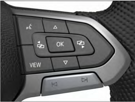
Fig. 11 Right-hand side of the multifunction steering wheel: controls for using the menus and information displays in the digital instrument cluster Pro version (variant 1).
