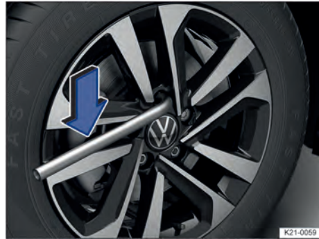
Fig. 257 Wheel change: Unscrew the wheel bolts with the wheel wrench.
