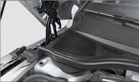
Fig. 260 Between the engine compartment and the windscreen: plenum chamber (illustration).
