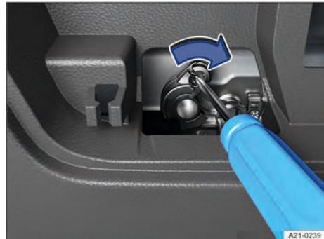
Fig. 72 In the boot lid: manual release mechanism for the boot lid.
