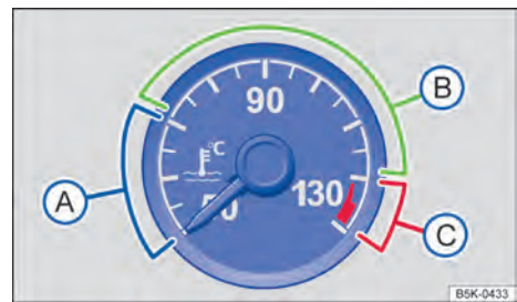
Fig. 21 Coolant temperature display in the analogue instrument cluster (schematic diagram).
