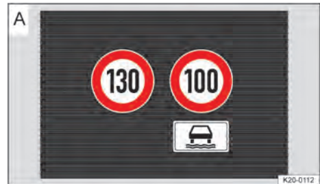
Fig. 28 On the instrument cluster display: example displays of the Dynamic Road Sign Display function.
