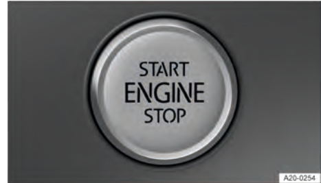
Fig. 120 In the lower section of the centre console: starter button for starting the engine.
