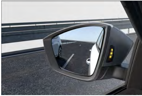
Fig. 152 In the exterior mirror housing: visual displays of the lane change system.
