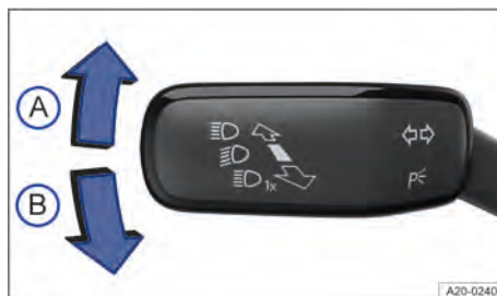
Fig. 96 On the left-hand side of the steering column: turn signal and main beam lever.
