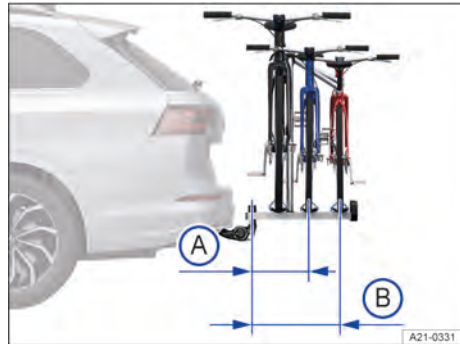
Fig. 193 Illustration of the maximum overhang on a bicycle carrier for two or three bicycles.
