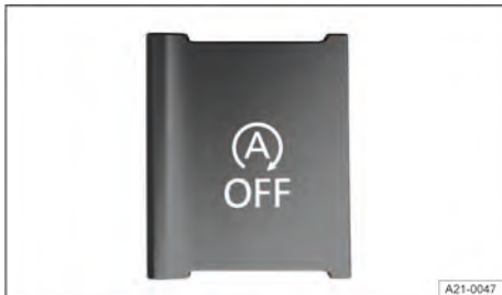
Fig. 122 In the lower part of the centre console: button for the start/stop system.
