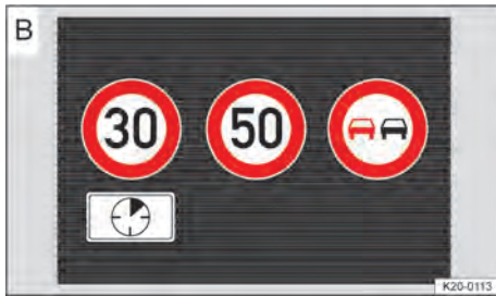
Fig. 29 On the instrument cluster display: example displays of the Dynamic Road Sign Display function.
