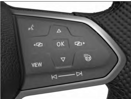
Fig. 12 Right-hand side of the multifunction steering wheel: controls for using the menus and information displays in the digital instrument cluster Pro version (variant 2).
