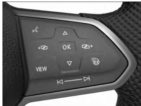
Fig. 16 Right-hand side of the multifunction steering wheel: buttons for using the menus and information displays in the analogue instrument cluster (variant 2).
