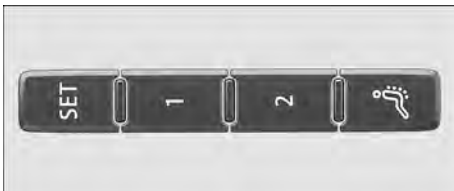
Fig. 93 On the outside of the driver seat: memory buttons.
