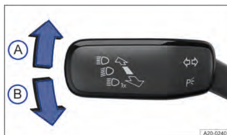
Fig. 99 On the left-hand side of the steering column: turn signal and main beam lever.
