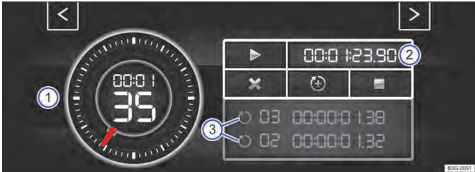
Fig. 24 On the Infotainment system display: lap timer with stopwatch, function button and lap times.
