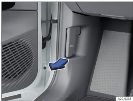
Fig. 228 In the footwell on the driver side: bonnet release lever (schematic diagram).
