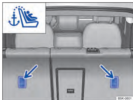
Fig. 52 On the back of the rear bench seat: anchor rings for the top tether.
