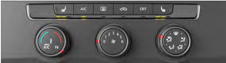
Fig. 111 In the upper section of the centre console: air conditioning block for the manual air conditioning system.
