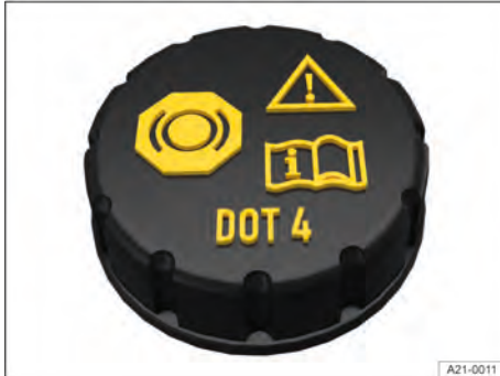
Fig. 238 In the engine compartment: cap of the brake fluid reservoir.
