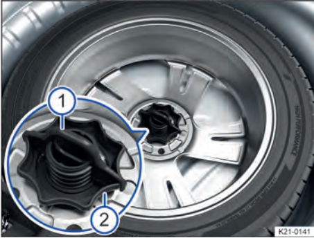
Fig. 253 In the luggage compartment: handwheel for securing the spare wheel.
