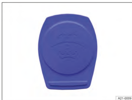
Fig. 231 In the engine compartment: washer fluid reservoir cap (illustration).
