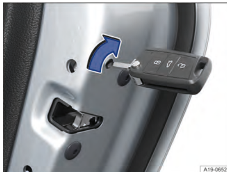
Fig. 62 In the front edge of the rear right-hand door: manually locking the vehicle with the vehicle key (illustration).
