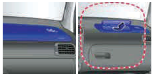
Location and deployment range of front passenger airbag
