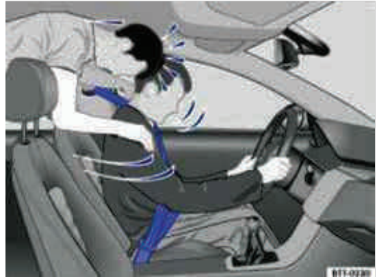
The unbelted rear passenger is thrown forward violently, hitting the driver wearing a seat belt.
